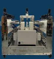
Also available as an upgrade to current BMP's, the Medusa is a hybrid system, with 10 automatically fed and 5 batch fed reactors. Suited to fibre-free or slurry feedstocks and covering both feeding regimes, the Medusa can perform versatile research particularly into microbial kinetics due to its many possible feedings configurations
