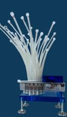
The Chimera innovates the analysis process by automatically reading CH₄ and CO₂ composition online, from a maximum of 15 individual reactors. It only requires a gas sample of 15ml, allowing for more frequent and holistic analysis, as well as maintaining functionality under low gas flow conditions such as standard BMP tests.
