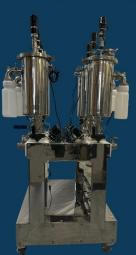
From our automatic range, the lobster model is equipped with six, 5 litre reactors (smaller options available). With an adjustable rate between 0 and 999 feeds a day, and the capability to use mixed fluid feedstocks from AD plants directly, the lobster can closely simulate the feed of an industrial AD plant.
