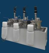
The Pegasus is our second batch-fed model, featuring 5/10L reactors. With up to 18% dry solid substrate having been used before, these larger capacity digesters enable the use of more fibrous and solid content that would be unsuitable for automatic feeding - as well being easier to operate with (less spillage when feeding).
