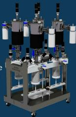
The Lobster-i model features 5 litre reactors (smaller options available), but with more flexibility for the feeding rate since each of the 4 reactors is equipped with its own feeder. This means 4 independent tests can be run simultaneously from the same machine. The Lobster and Lobster-i can both later be converted to multi-stage systems.
