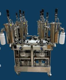
Boasting many possible configurations, the Black Swan is our most comprehensive model. With four 1st stage and four 2nd stage reactors (+optional additional stages), and 4 auto-feeders, the Black Swan allows you to compartmentalise the AD process by manipulating each stage through temperature control and HRT.
