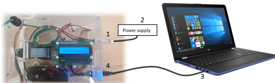
Figure 19. Arduino connexions. The numbers show the connection procedure order to be followed.
