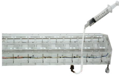
Figure 8. (3.1) Gas flow meter levelled, (3.2) Operational position of the drain pipe, (3.4) Gas flow meter calibration.
