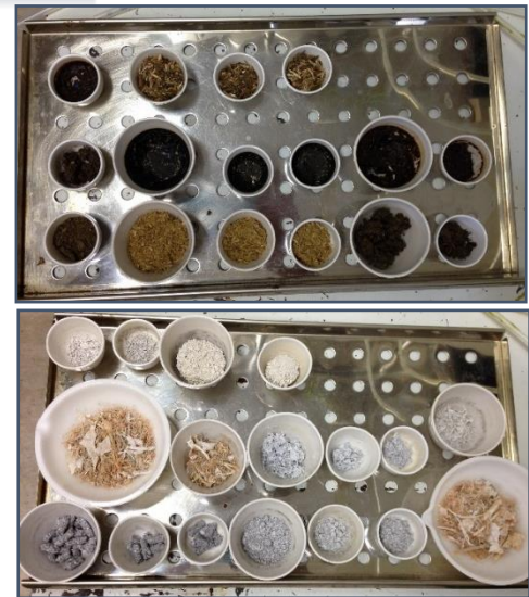
Figure 12. Crucibles with samples before and after Total solids and volatile solid analysis.
